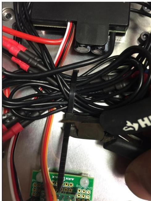
6. Disconnect all Motor and ESC wires.
