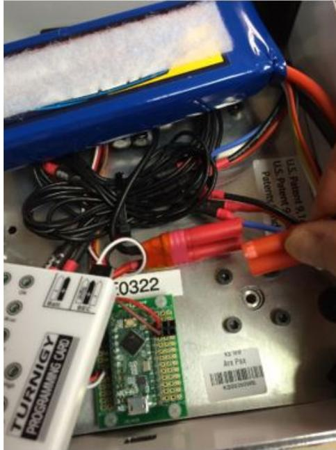
4. Use the up/down and left/right arrows at the base of the card to choose your desired settings. Press OK to program. After blue "connecting light turns off, unplug the battery. For reference, the settings that came on the Whitebox are shown below.
