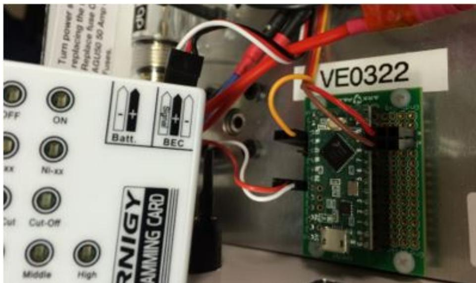
3. Plug in battery. The ESC will beep. Wait for a moment and the settings will light up on the program card.
