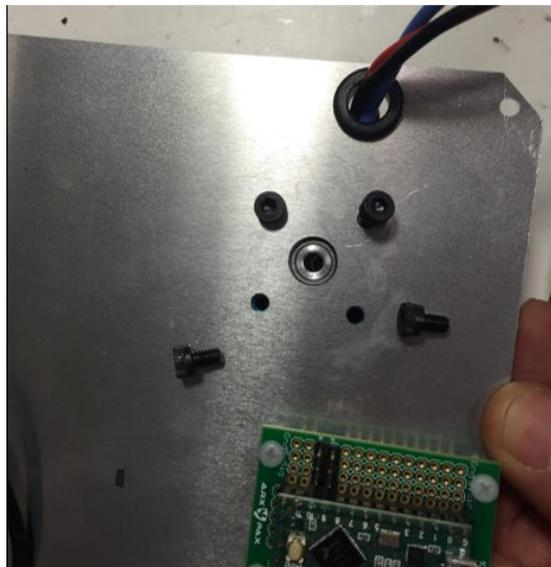
8. Unscrew the nylon hex nuts to separate the Teensy Microcontroller from the chassis.
